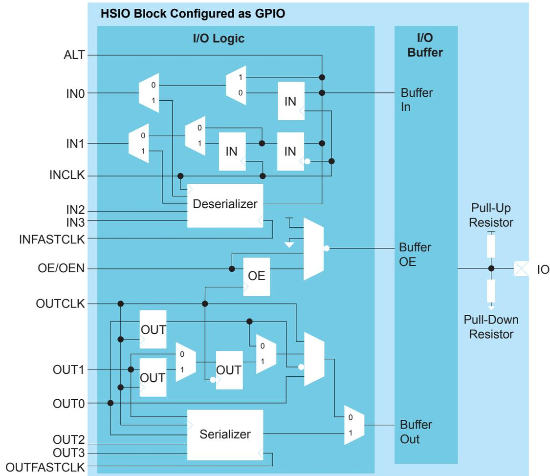
Table 12: HSIO Block Configured as GPIO Signals (Interface to FPGA Fabric)
