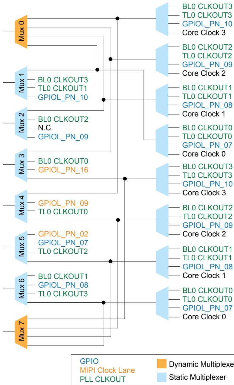
Figure 11: Clock Sources that Drive the Multiplexers: Right
