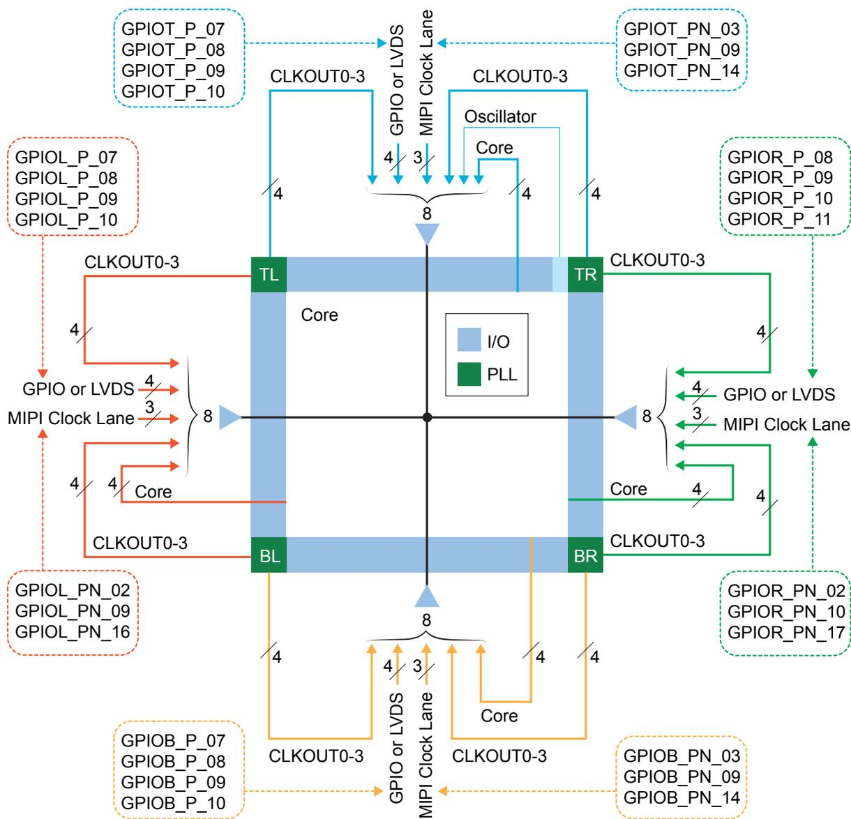
Numerous clock sources feed the global network. These signals are multiplexed together with static and dynamic clock multiplexers.
