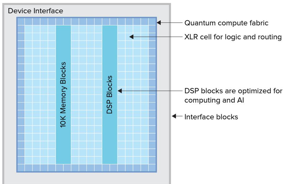
Interface blocks include GPIO, LVDS, PLL and MIPI lane I/O.
