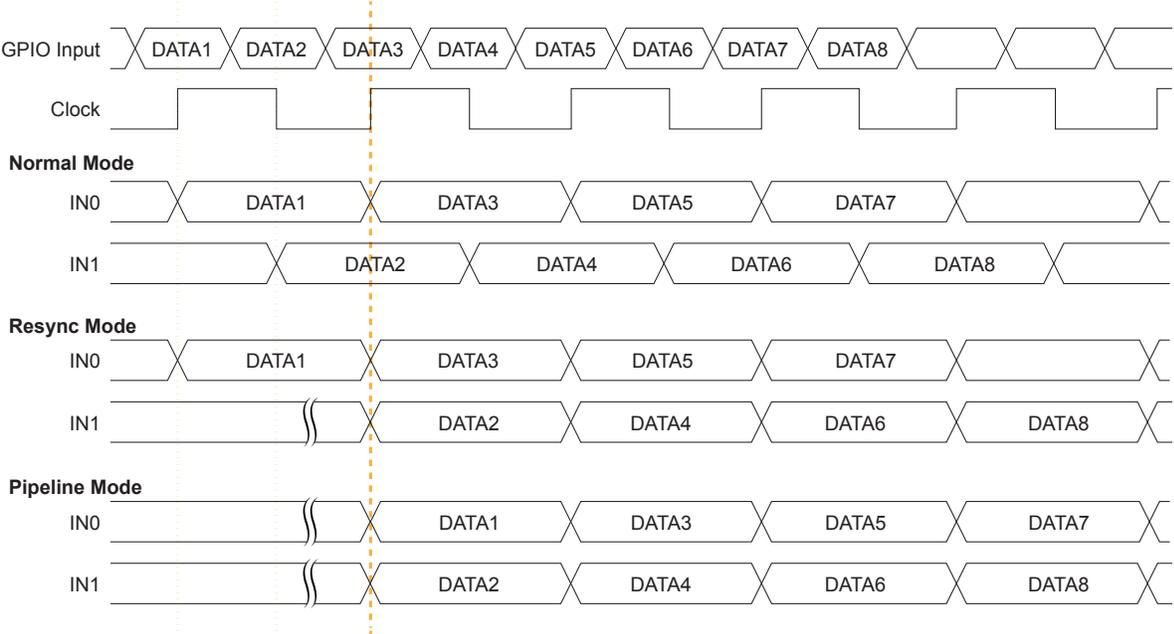
In resync mode, the IN1 data captured on the falling clock edge is delayed one half clock cycle. In the Interface Designer, IN0 is the HI pin name and IN1 is the LO pin name.
