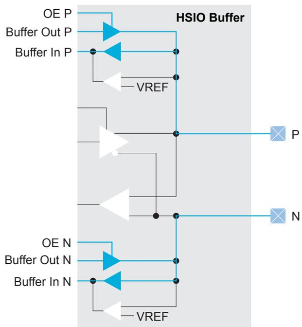
When using an HSIO with the HSTL or SSTL I/O standards, you must configure an I/O pad of the standard's input path as a VREF pin. There is one programmable VREF per I/O bank.
