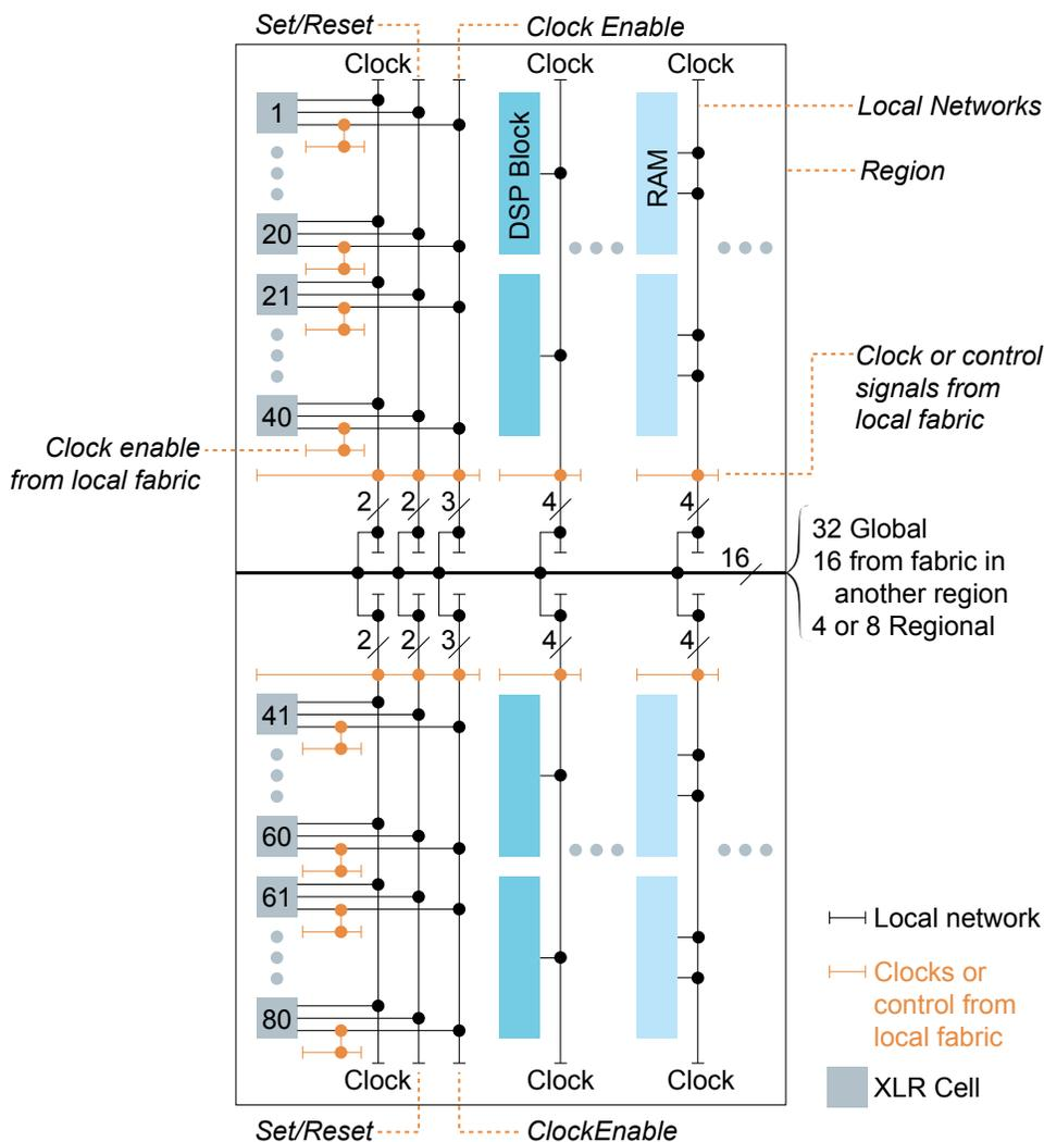
There are 16 signals that can feed the local networks. These signals can come from several sources:
