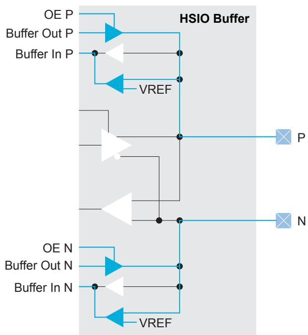
When using an HSIO with the differential HSTL or differential SSTL standard, you must use both GPIO resources in the HSIO. You use the core interface pins associated with the P resource.
