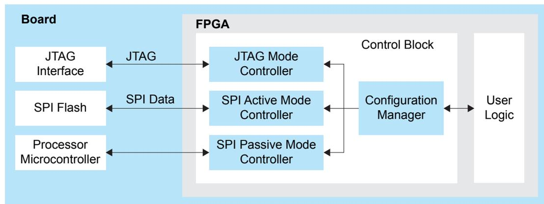
In active mode, the FPGA controls the configuration process. The configuration clock can either be provided by an oscillator circuit within the FPGA or an external clock connected to the EXT\_CONFIG\_CLK pin. The bitstream is typically stored in an external serial flash device, which provides the bitstream when the FPGA requests it.
