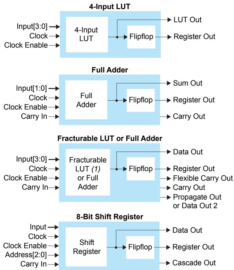
1. The fracturable LUT is a combination of a 3-input LUT and a 2-input LUT. They share 2 of the same inputs.
