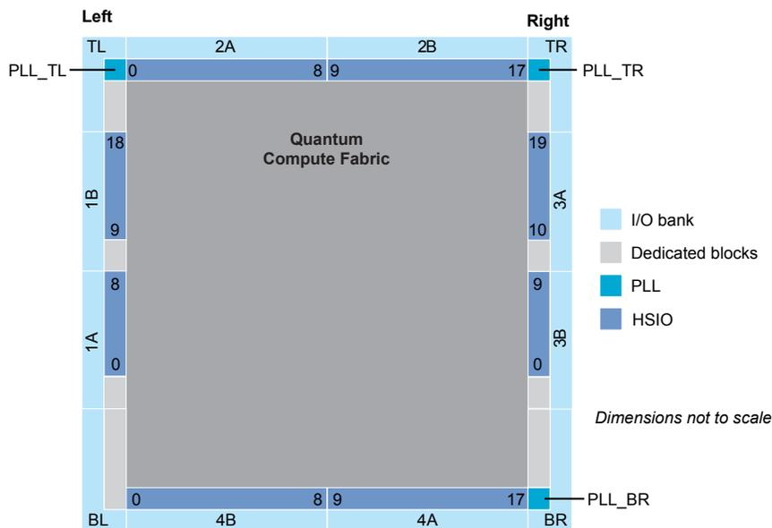
Figure 44: Floorplan Diagram for F225 and F256 Packages
