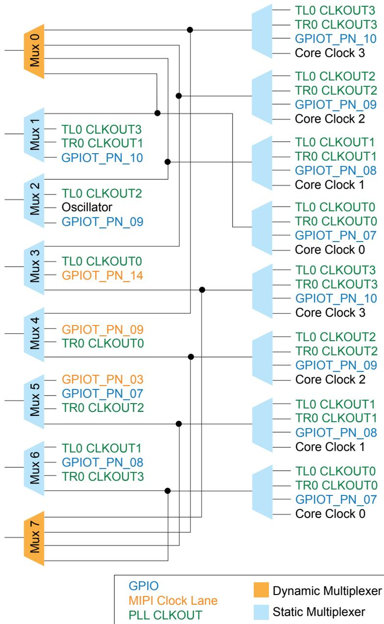
Figure 9: Clock Sources that Drive the Multiplexers: Bottom
