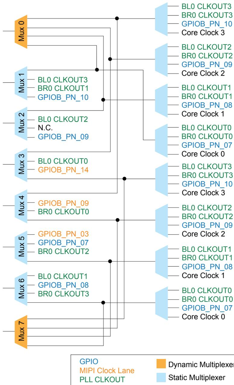
Figure 10: Clock Sources that Drive the Multiplexers: Left
