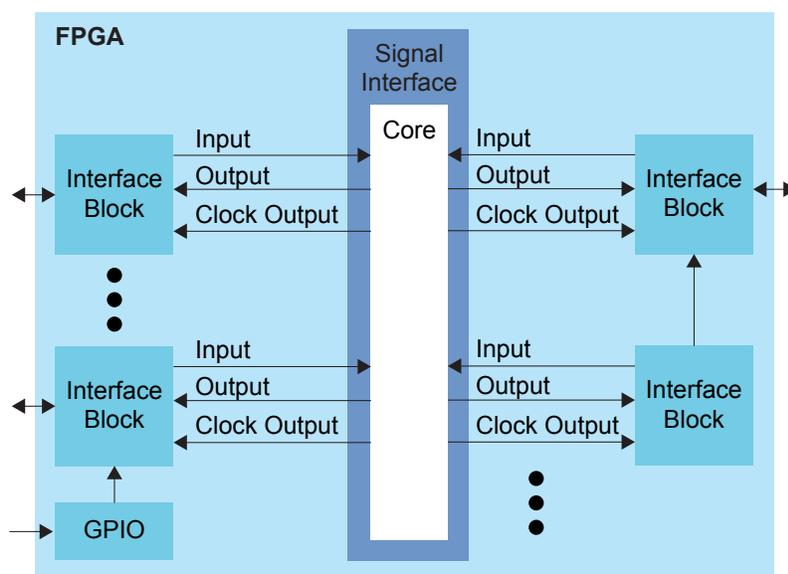
GPIO blocks are a special case because they can operate in several modes. For example, in alternate mode the GPIO signal can bypass the signal interface and directly feed another interface block. So a GPIO configured as an alternate input can be used as a PLL reference clock without going through the signal interface to the core.
