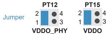
Figure 10: Connect Pins 1 and 2 on PT12 and PT15
