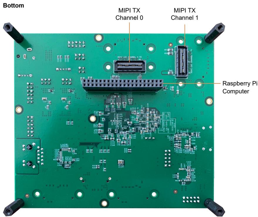
The Trion® T120 BGA324 Development Board provides four 0.8 mm high-speed ground plane sockets for the MIPI CSI-2 interface and two 0.8 mm high-speed ground plane sockets for the LVDS transmitters and receivers. It has two sockets to connect PMOD-compatible peripherals. Additionally, it has a 0.5 mm high-speed connector for additional I/O pins and one 40-pin header for connecting to a Raspberry Pi computer.
