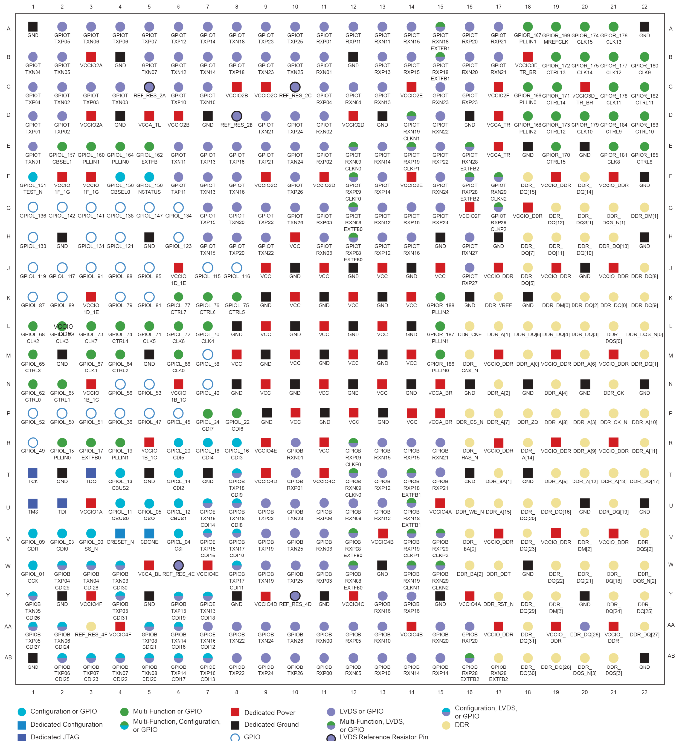
Figure 41: 484-Ball FBGA Pinout Diagram
