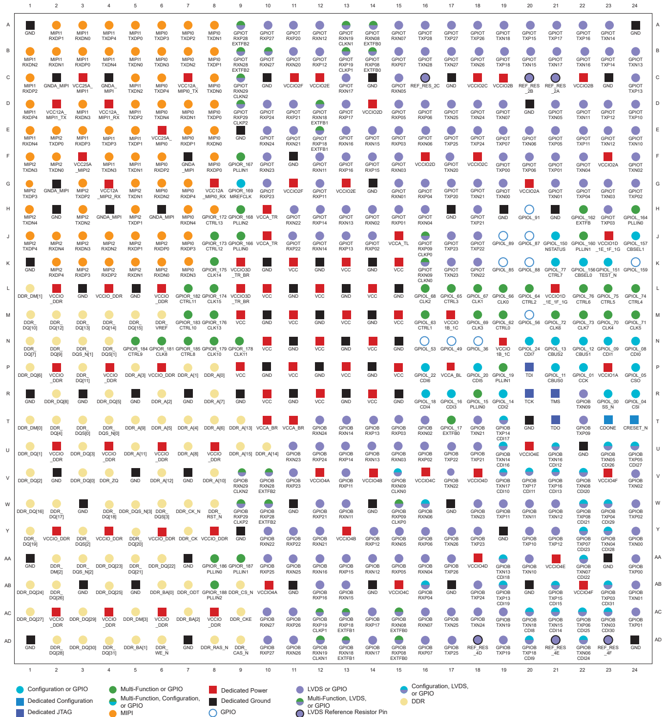
Figure 45: 576-Ball FBGA Pinout Diagram
