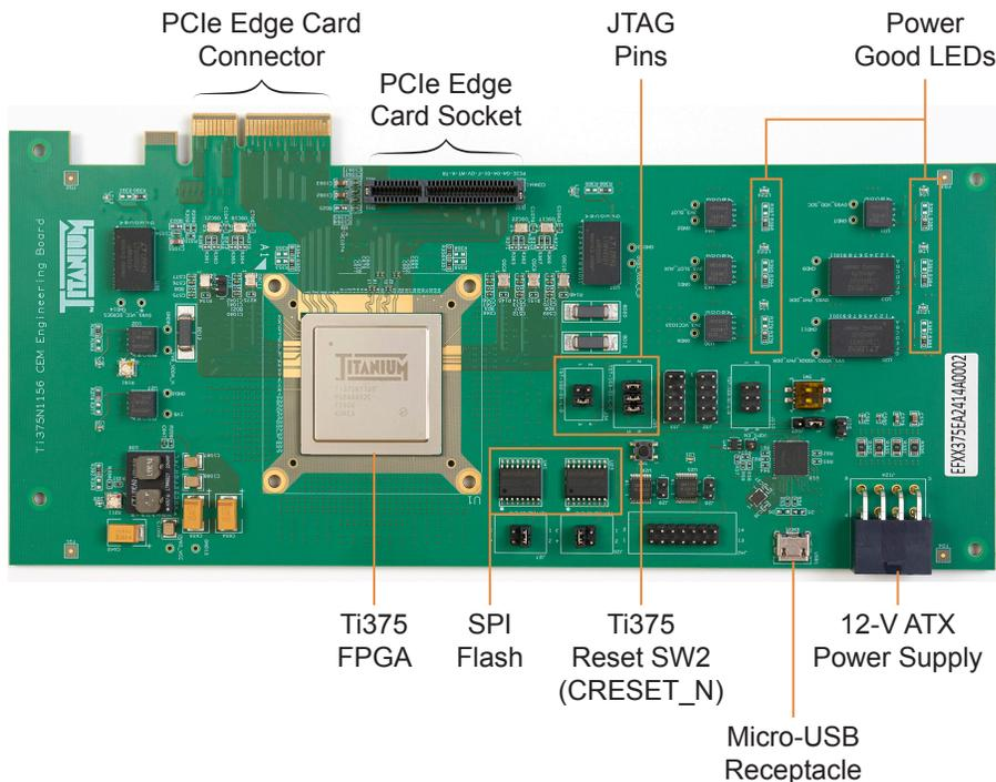
The board includes a micro-USB port for the FTDI interface. The FTDI FT2232H module supports the following interfaces:
