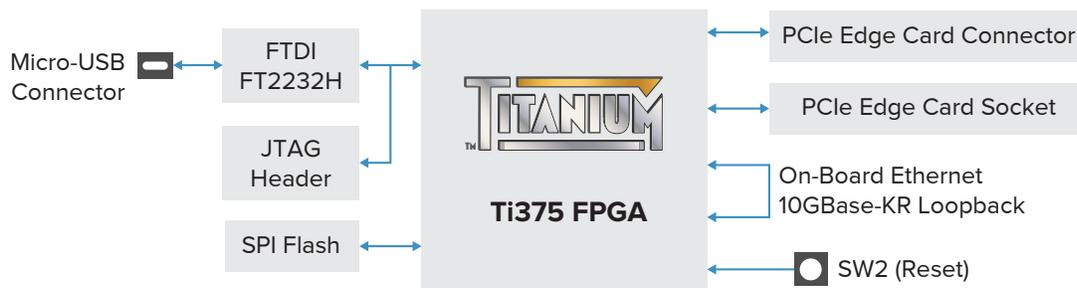
The main purpose of this board is to demonstrate the PCIe Gen4x4 capability. However, the board also has a direct connection between the non-PCIe transceiver banks, which can be used for an Ethernet 10GBase-KR loopback. However, Efinix will not be providing an example design to demonstrate that functionality.
