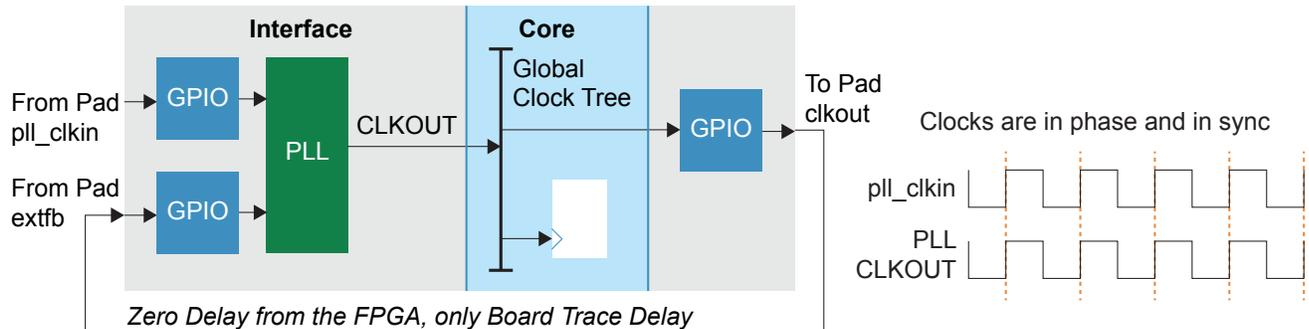
When the PLL is in external feedback mode, the compensation delay is equal to GPIO\_IN plus the clock network delay plus GPIO\_CLK\_OUT.
