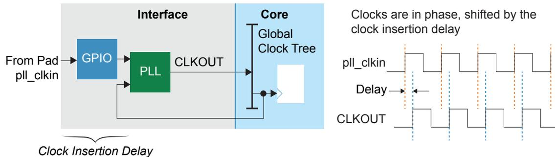
When the PLL is in core feedback mode, the compensation delay is equal to the clock network delay.
