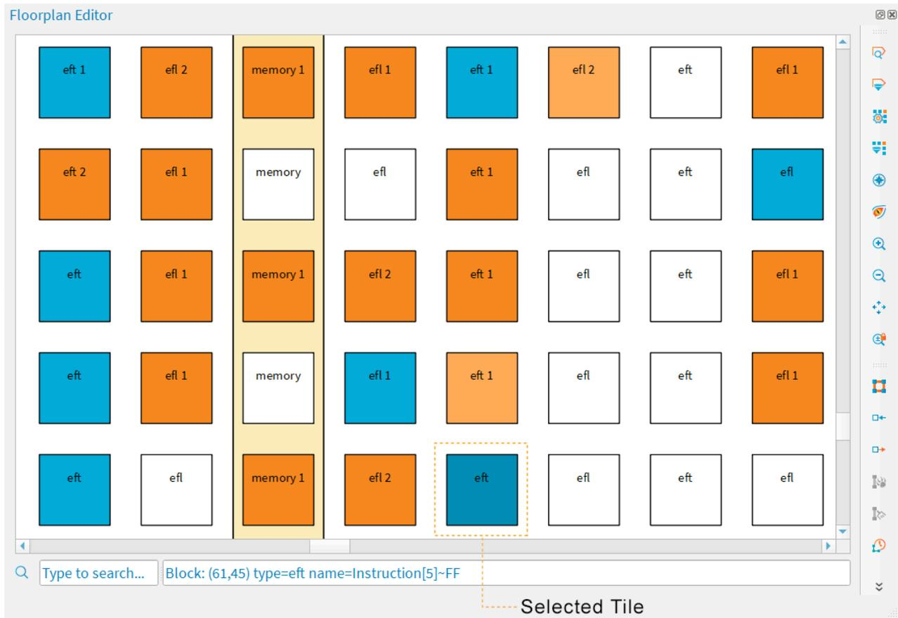
Notice that some tiles in the floorplan have a number. This number indicates how many routing lines are used in that tile. A tile used for logic (blue) can also be used as routing (indicated by the number). Orange means a tile is only used as routing.
