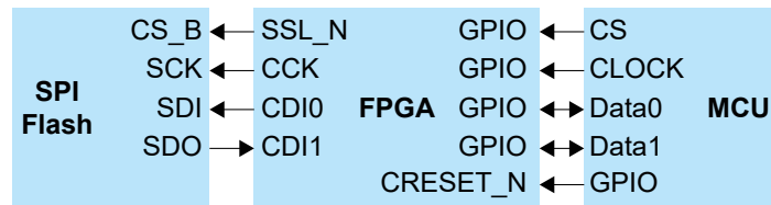
Figure 24: FPGA Configured with SPI Bus Connections to SPI Flash and GPIO Emulated MCU SPI Bus Connections to MCU
